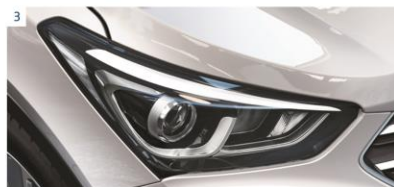
2. Redesigned Radiator Grille 3. Projection Type Headlamp
